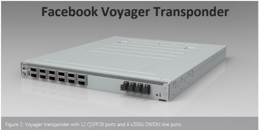
Figure 2: Voyager transponder with 12 QSFP28 ports and 4 x200G DWDM line ports.
